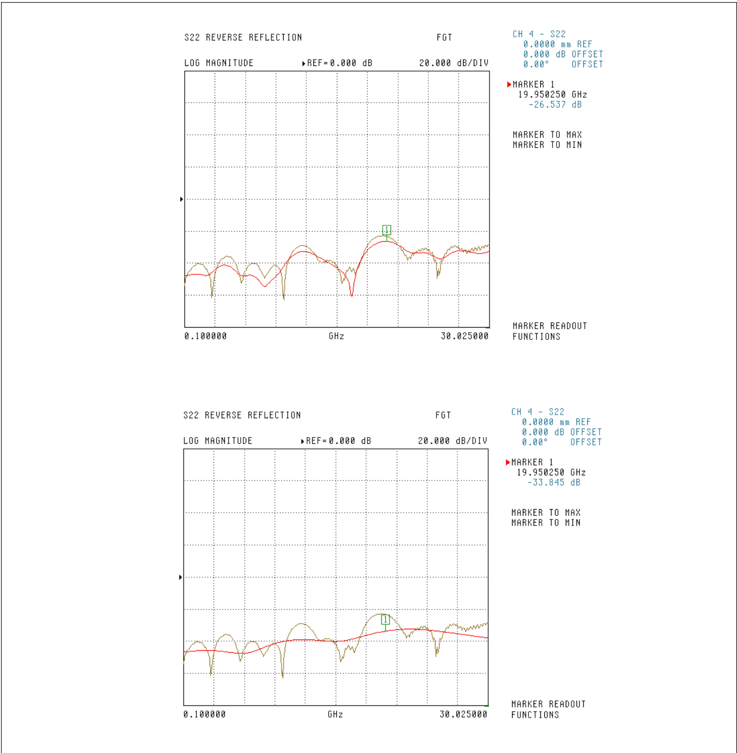
Figure 19. The reflection coefficient of our standard delay line is shown here without gating (light trace) and with gating (dark trace). In the top graph, a rectangular gate width matched to the adapter length was used and the results are reasonable (aside from some low frequency and high frequency inflections). In the bottom graph, a less well-defined window is used. While edge inflections are removed, much valid information is as well since there is physically little distance between adapter and DUT.
